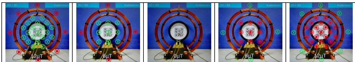
Fig. 3. Temporal development of the magnetic field according to the corresponding film strip in Fig. 1. The green crosses and red dots symbolize magnetic field lines directed into or out of the plane, respectively.
